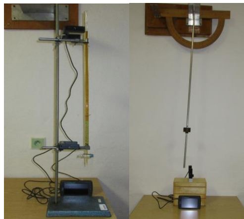
Figure 8. Determination of kinematic viscosity and the physical pendulum period
